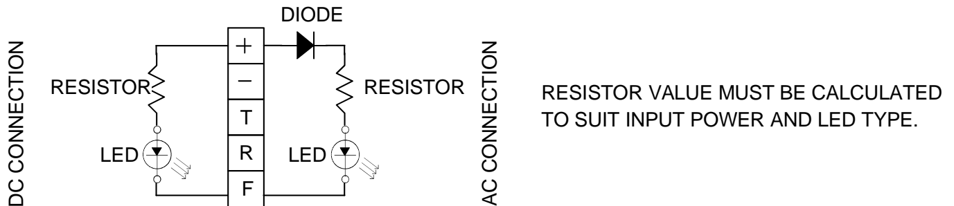
FIG. 3: FLASH OUT CONNECTIONS TO EXTERNAL LED
