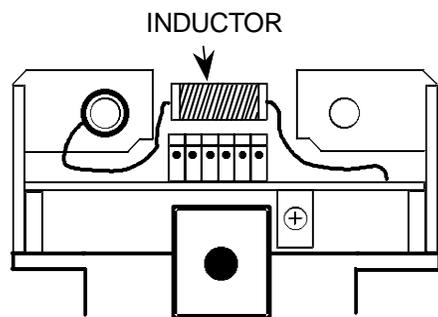
SOLDER ONE END OF INDUCTOR INTO PAD MARKED "BAR" ON RIGHT SIDE OF SENSOR. CLIP WIRE FROM RING TERMINAL, REMOVING IT FROM SENSOR AND CONNECT IT TO OTHER END OF INDUCTOR.
