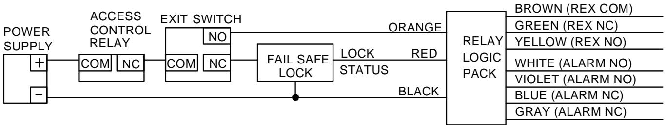
"LOCK STATUS" WIRE MUST OUTPUT +V WHEN LOCK IS SECURE
