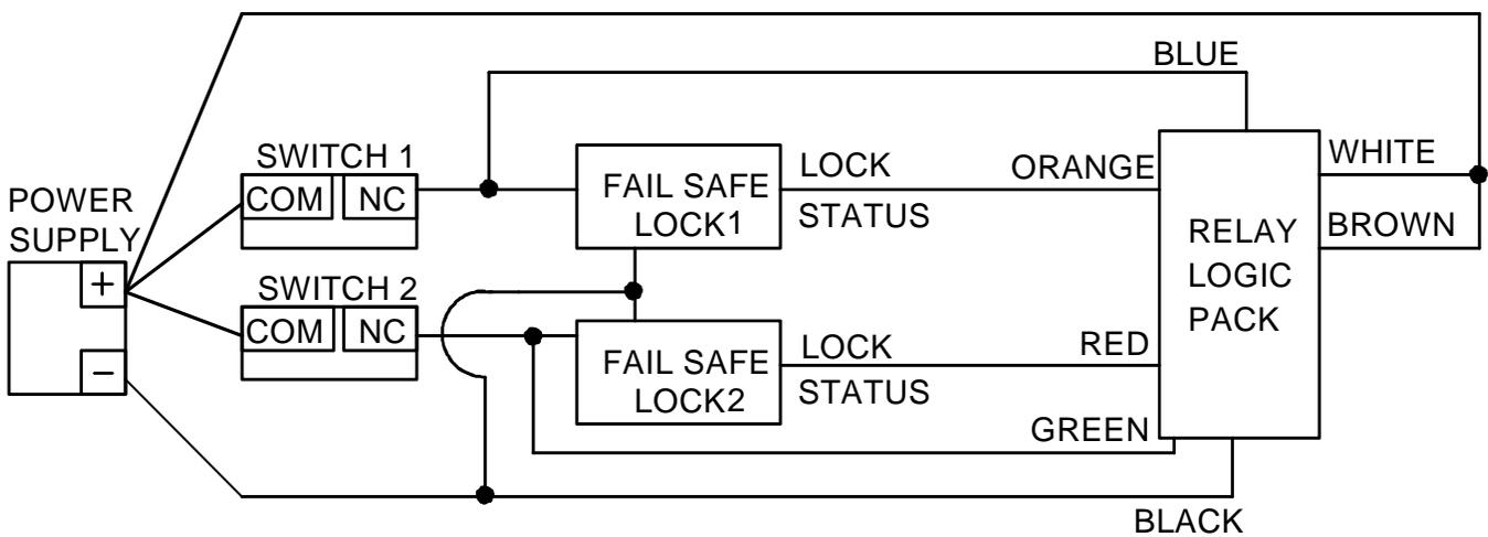
"LOCK STATUS" WIRE MUST OUTPUT +V WHEN LOCK IS SECURE
