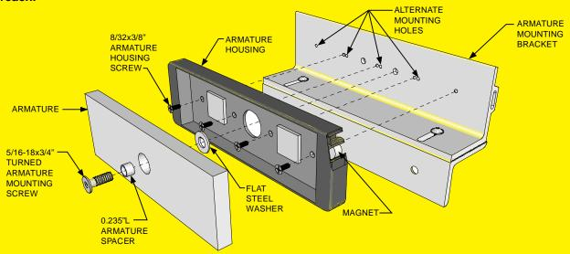
NOTE: For locks ordered with the DSM or HSM option, please verify that two magnets are installed inside the armature housing.
